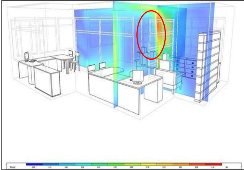
HVAC “hotspots” airflow problems
